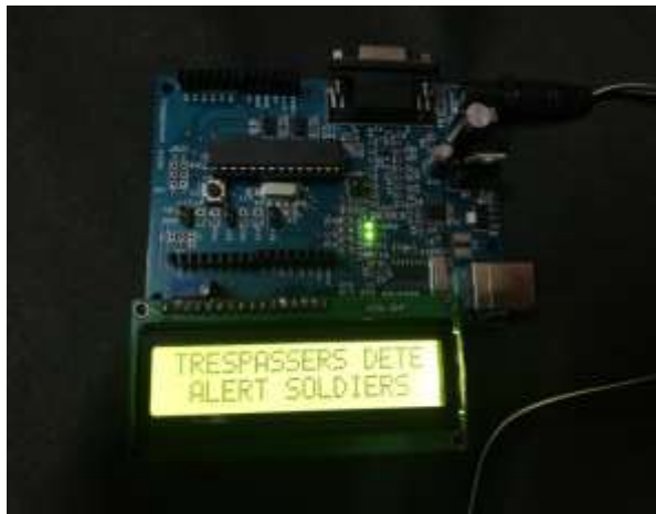
Fig. 4. Trespasser detection information displayed in LCD display
