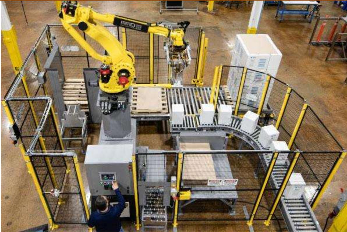
Fig. 7. A six-axis robot in a safety fence (Source: [www.mmci-automation.com/palletizing-safety](http://www.mmci-automation.com/palletizing-safety)).
