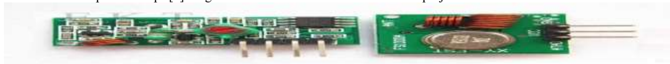
Figure 2: Transmitter and Receiver with RF Module Pin Diagram [1].
