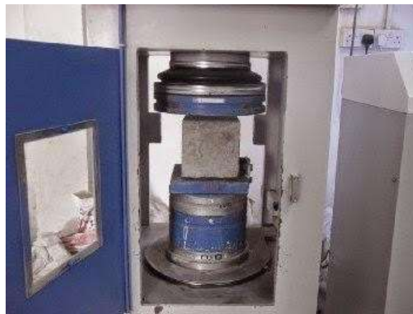
Fig.4 Compression test on concrete cube in progress
