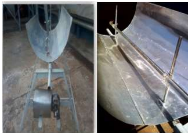
Figure 2: Complete assembly of the parabolic trough
