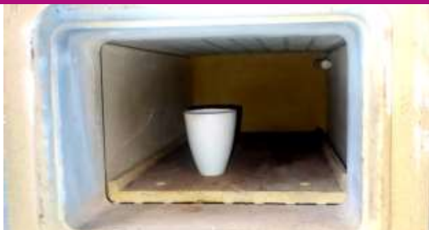
Fig.4. Incineration of a mixture of non-magnetic fraction of concentrator waste and lime in a muffle furnace
