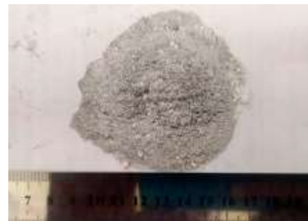
Fig.3. An example of a shale made with a mixture of concentrator waste and lime
