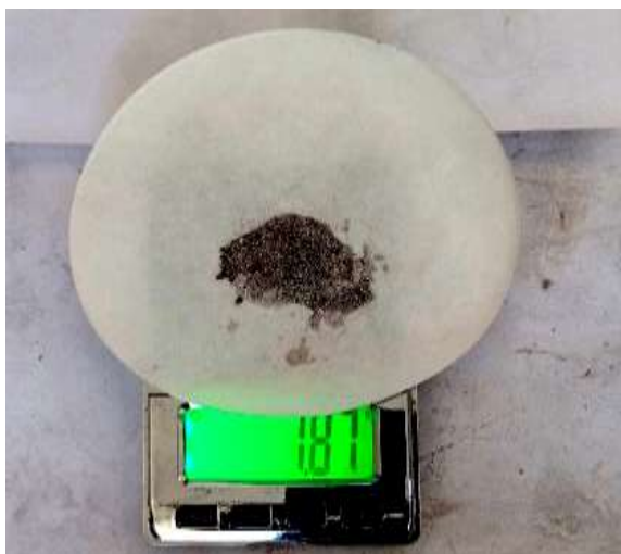
Fig.5. The magnetic fraction of the product formed after lime is added to the non-magnetic part of the concentrator waste
