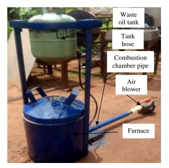
Fig. 2.2: The prototype waste oil burner connected to a furnace
