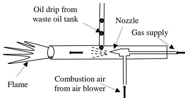
**Fig. 2.1: Schematic diagram of the waste oil burner**
