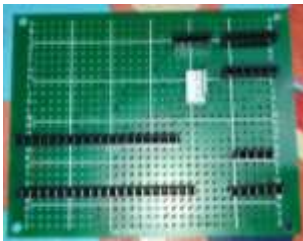
Figure 13. View from the top of the dot PCB after the pin header is installed
