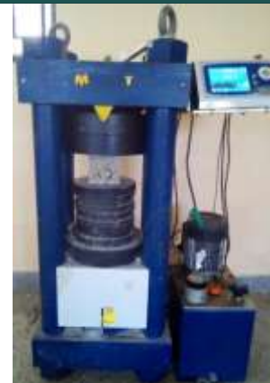
Fig. 13. MATEST CO89PN140 compressive test machine
