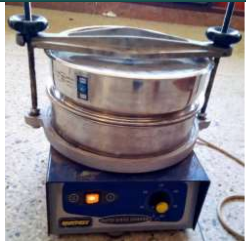
Fig. 6. MATEST A060 - 01 Auto Sieve Shaker
