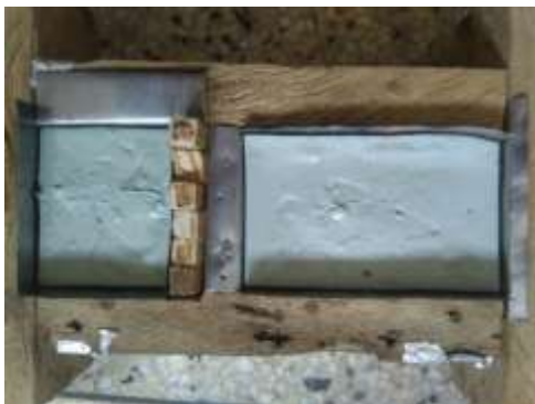
Fig. 4. Wooden mould containing molten plastic left to cool
