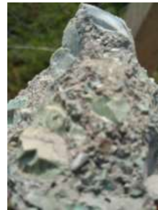
Fig. 14. Cubic concrete specimen after failure
