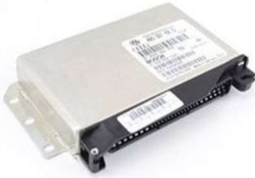
Fig. 16. Transmission control module bus
