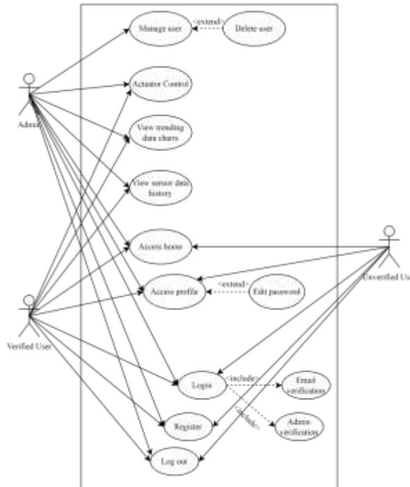
Fig. 4. Use Case Diagram of System
