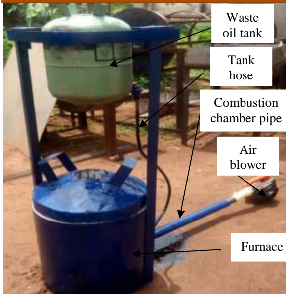
Fig. 2.7: The prototype waste oil furnace connected to a burner
