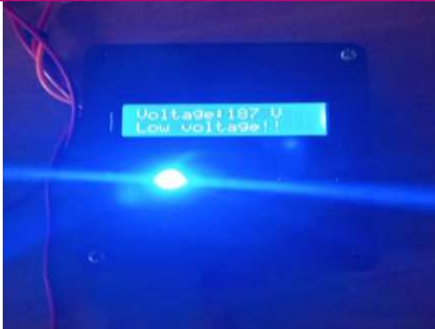
Figure 6: showing what happens when the voltage is low
