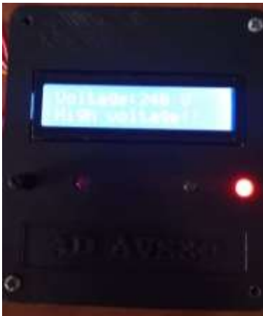
Figure 8: showing what happens when the voltage is above range
