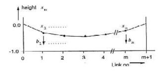
Consider a hanging chain of m + 1 light links with fixed ends at height  $x_0 = x_{m+1} = 0$ . It could be the supporting chain for the Clifton suspension bridge in Bristol, shown  $\Rightarrow$ There is unit tension in the chain, the links are of unit
