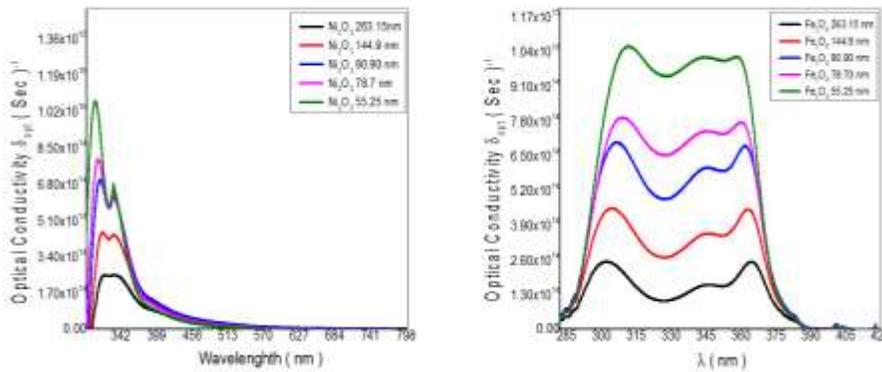
Fig(4) the relation between optical conductivity and wavelngths of  $\text{Ni}_2\text{O}_3$  and  $\text{Fe}_3\text{O}_4$  samples in different thickness
