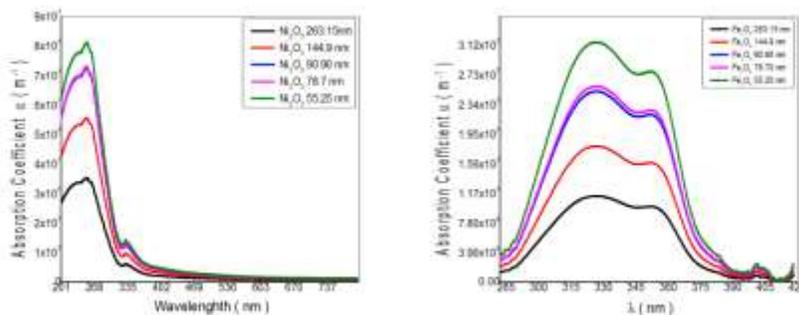
Fig(2) the relation between absorption coefficient and wavelengths of Ni<sub>2</sub>O<sub>3</sub> and Fe<sub>3</sub>O<sub>4</sub> samples in different thicknesses
