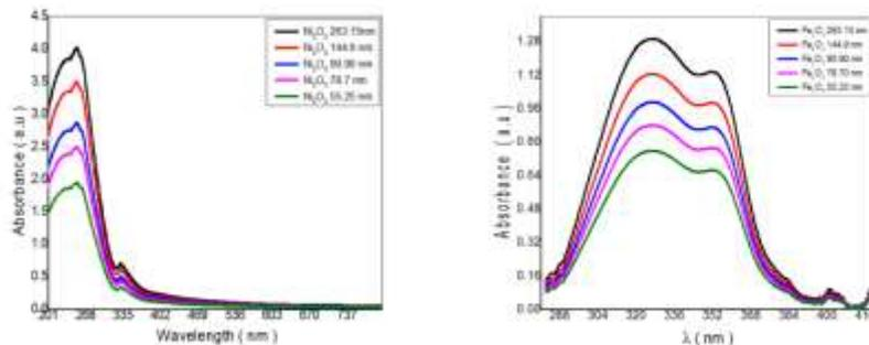
Fig(1) relation between absorbance and wavelengths Ni<sub>2</sub>O<sub>3</sub> and Fe<sub>3</sub>O<sub>4</sub> samples in different thicknesses
