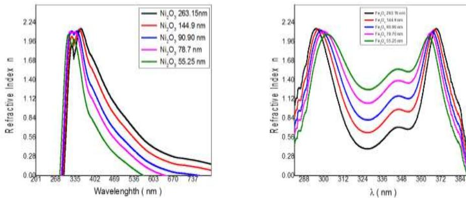
Fig(3) the relation between refractive index and wavelngths of  $\text{Ni}_2\text{O}_3$  and  $\text{Fe}_3\text{O}_4$  samples in different thicknesses
