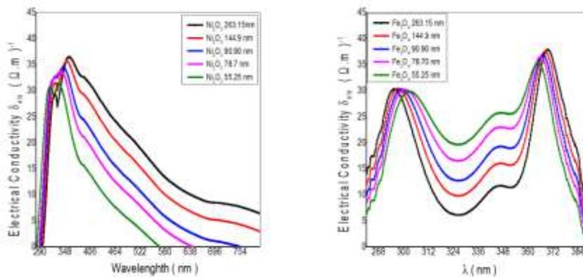
Fig(5) the relation between electrical conductivity and wavelngths  $\text{Ni}_2\text{O}_3$  and  $\text{Fe}_3\text{O}_4$  samples in different thickness
