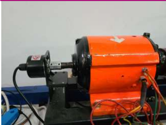
Fig. 4 Rotary Encoder coupled to SRM's shaft
