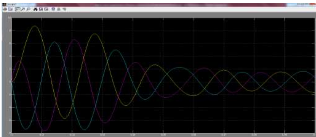
Figure 4. Graphs of changes in time of current forces passing through the stator windings during the start-up period of an asynchronous motor
