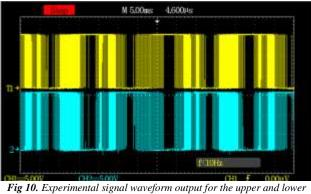
Fig 10. Experimental signal waveform output for the upper and lower legs
