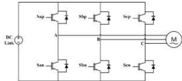
Fig 2. Skema three-phase inverter
