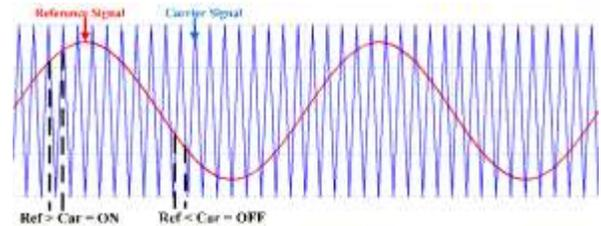
Fig 6. Comparison of reference and carrier signal waveform
