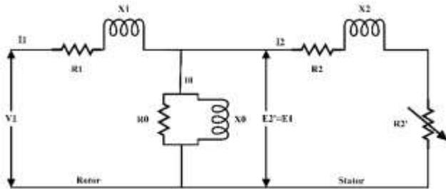
Fig 1. Asynchronous motor schematic circuit
