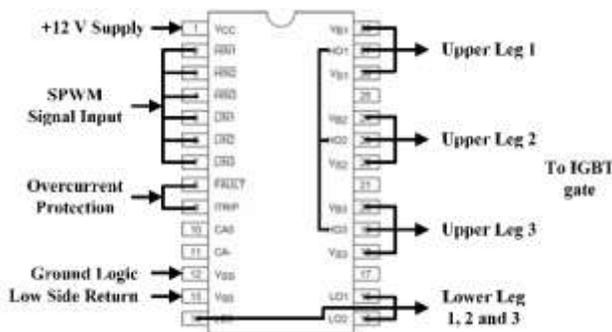
Fig 5. IR2132 driver schematic circuit
