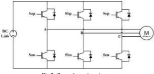
Fig 2. Skema three-phase inverter
