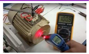
Fig 12. Speed measurement of the prototype
