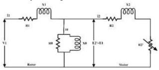
Fig 1. Asynchronous motor schematic circuit
