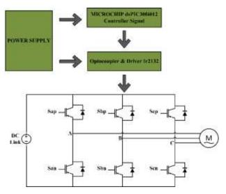
Fig 7. Hardware block diagram
