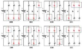
Fig 3. Three-phase inverter switching configuration
