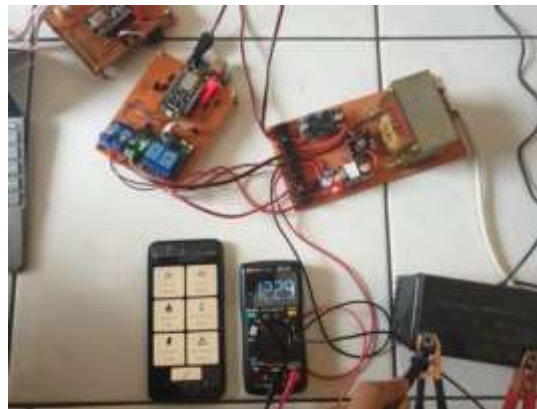
Fig. 5. Voltage sensor test circuit.
