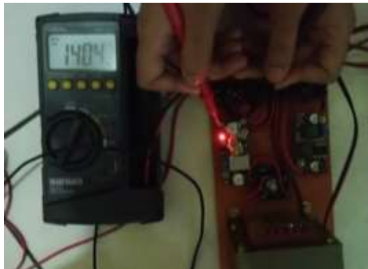
Fig. 3. The output voltage reading of the accumulator charger.
