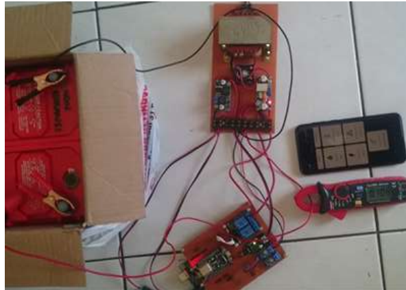
Fig. 6. Current sensor test circuit.
