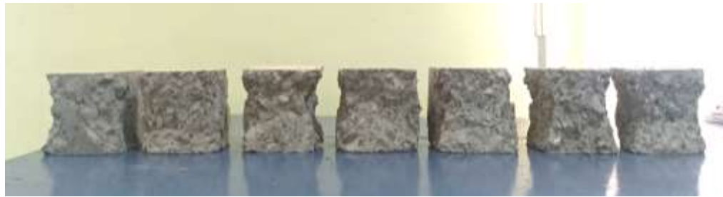
Figure 4. The general post-test appearance of cubic samples made of ordinary cube samples
