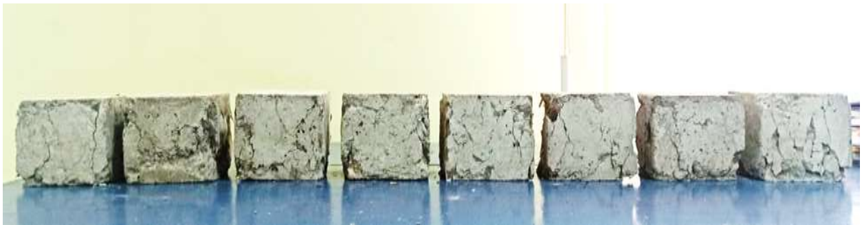
Figure 5. The general post-test appearance of cubic samples made of fibro-concrete
