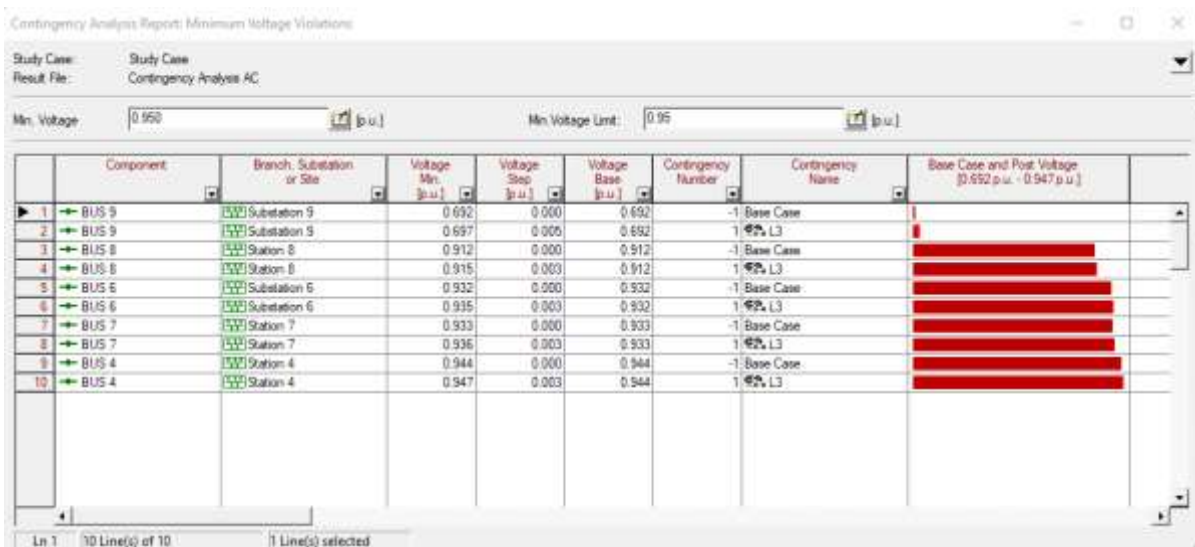
Figure 8: Contingency Analysis Report: Minimum Voltage Violations
