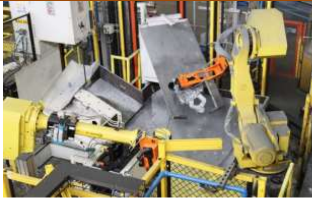
Fig 1. General Motors pick and place robot in aluminum die casting foundry. Source [5].
