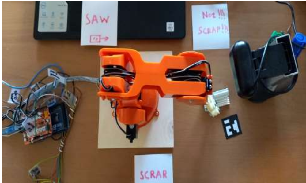
Fig 9. Robot from pick part to camera vision system.
