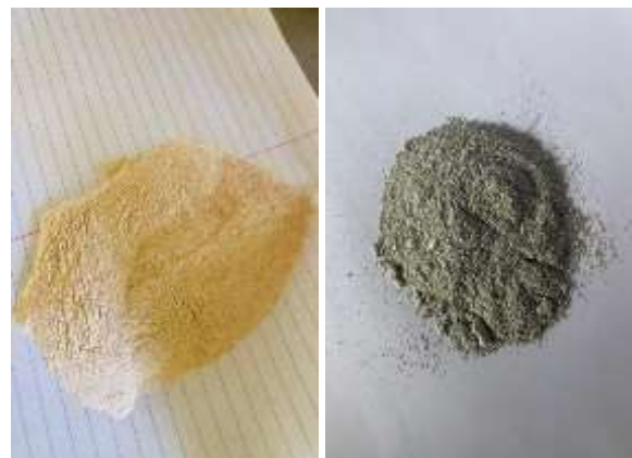
Fig. 3.2 Powdered eggshells after grinding and Eggshell powder after heating at 450^\circ\text{C} for 2 hours
