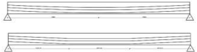
Fig.2. A graphical illustration of the tendons profile employed in the guideway girder.
