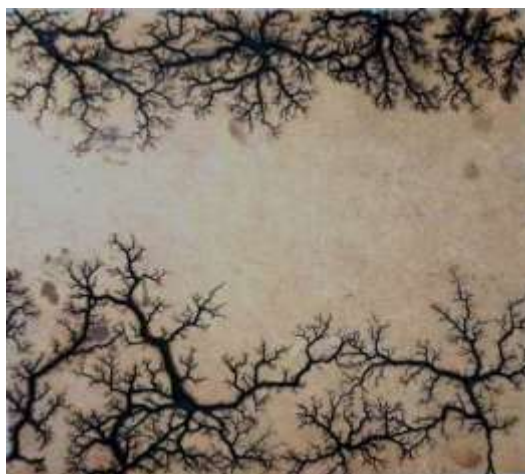
Fig.8. Electric Plasma Arc Ablation Response on a Fine Wood Powder Sheet.
