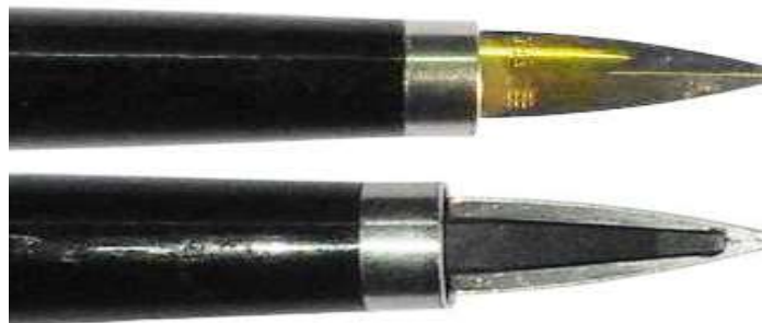
Fig.5. Modified Fountain Pen for Electrolytic Sketching Application
