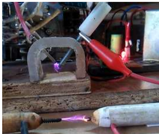
Fig.6A. Narrow gap of spark-gap gadget gives high intensity arc
