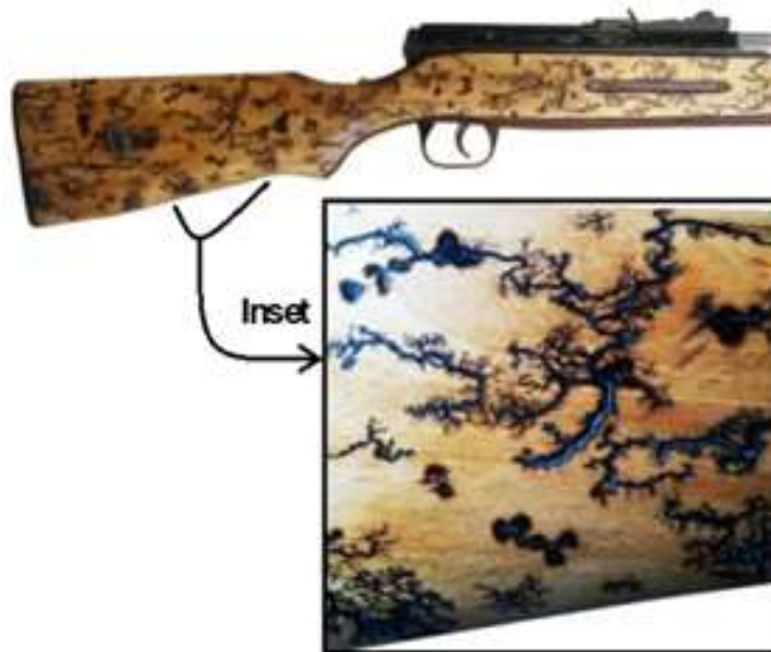
Fig.9. Electric Plasma Arc Ablation Pattern Generation on Air Gun Stock.
