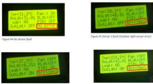
Figure 46 Sensor 1 Fault (Indoor light sensor error)
