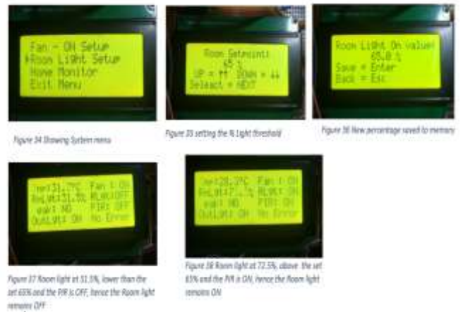
Figure 6: Reading the Medical Room Light Level and Tuning on the Medical Room Light
