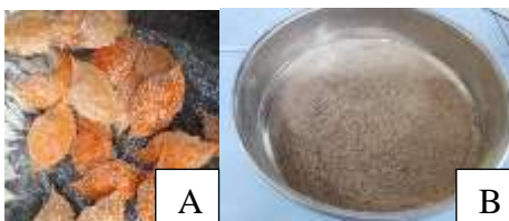
Figure 1. Results of the crab shell grinding process. (A) Crab shells before grinding. (B) Crab shell powder that has been ground with a grinder machine and sieved with a 100 mesh sieve.
