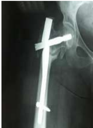
Hardware fracture on a non-union fracture
