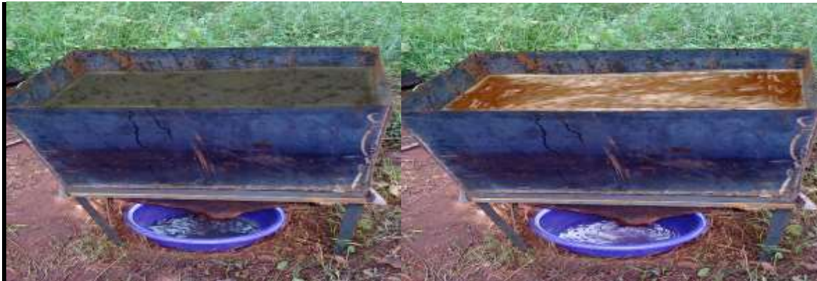
Fig. 1. Experimental Setup of Sand Drying Bed for Agricultural Sludge and Industrial Sludge
