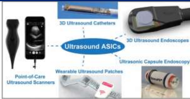
Figure 1: Examples of emerging medical ultrasound imaging devices (clockwise from the left): a hand-held point-of-care ultrasound scanner (image courtesy of Butterfly Network) [11]; a 3D intra-cardiac imaging catheter [9]; an artist’s impression of a 3D transesophageal ultrasound probe [14]; a pill-shaped ultrasonic endoscopy device (image courtesy of Univ. of Glasgow) [2]; an artist’s impression of a wearable ultrasound patch (image courtesy of ULIMPIA project)
