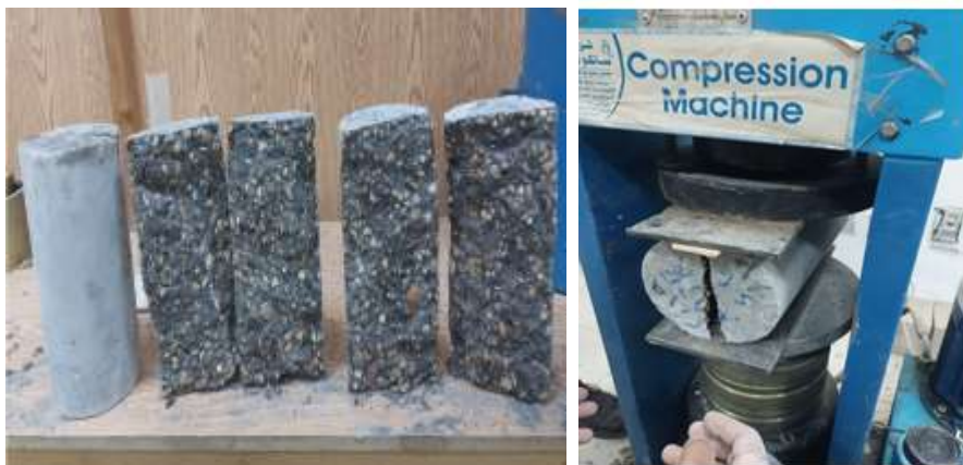
Figure 18. Failure models for specimens of reference and pozzolanic concrete under indirect tensile by compression machine
