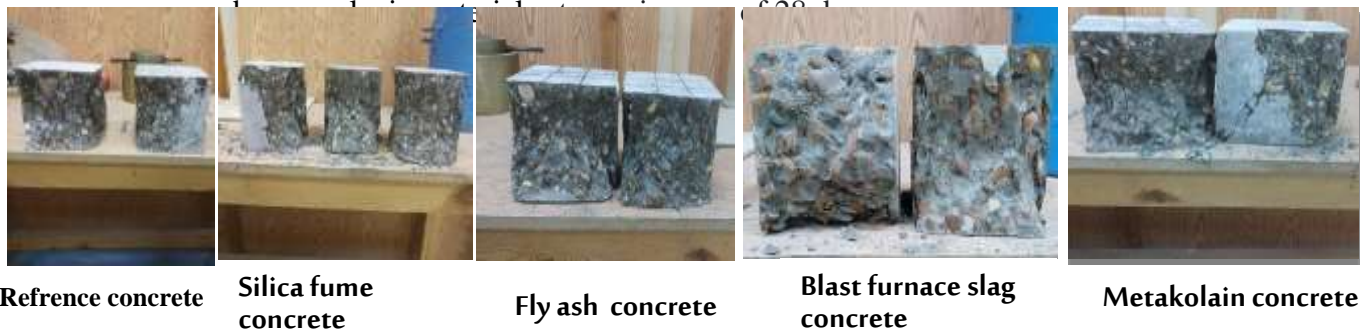
Figure 10. Failure models for specimens of refrence and pozzolanic concrete under axial compression
