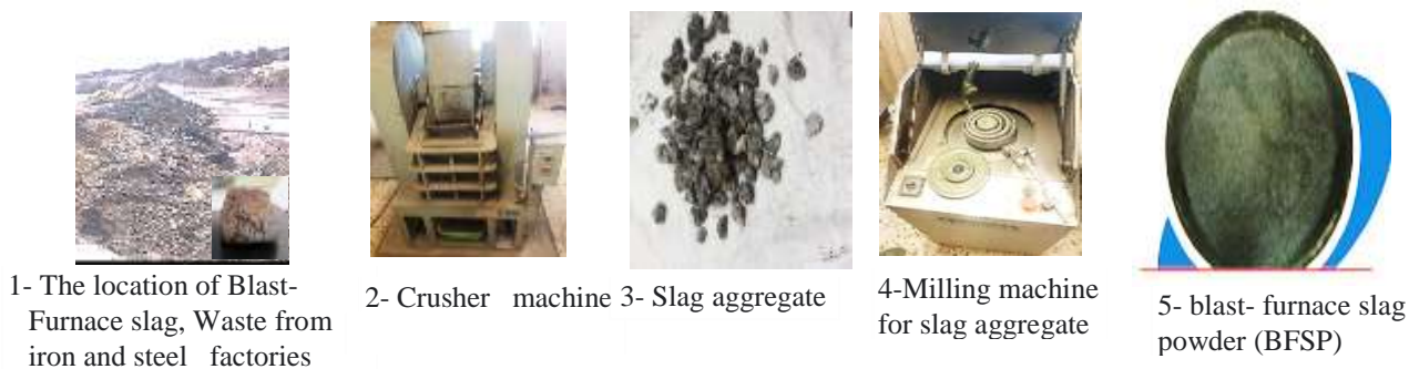
Figure 4. Shows the stages of preparing blast-furnace slag powder (BFSP)
