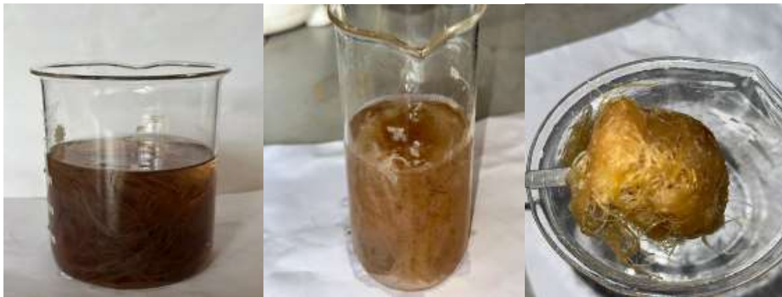
Fig. 4 Extracted fiber washed with distilled water
