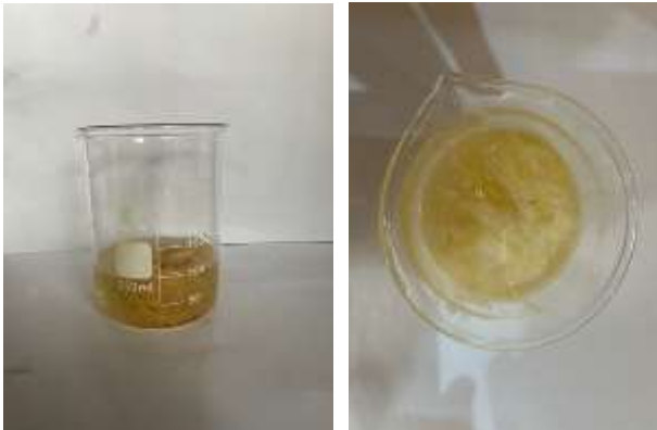
Fig. 7 Bleaching of the extracted plantain peduncle fiber in hydrogen peroxide
