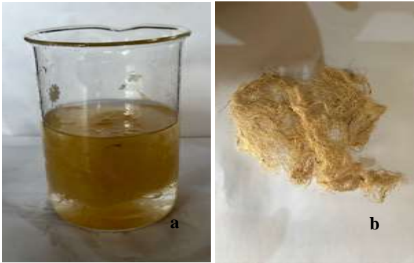
Fig. 6 Mercerized Fiber (unbleached) washed (a) in distilled water and dried (b)
