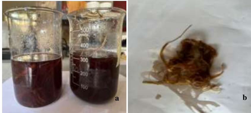
Fig. 3 Fibers extracted using 20% Sodium hydroxide solution
