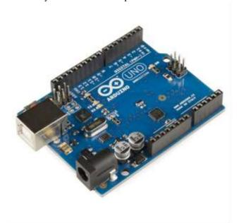
Arduino Uno can be powered through a USB connection or an external power supply. The voltage range is typically 7-12V. Arduino Uno is programmed using the Arduino IDE (Integrated Development Environment), which uses a simplified version of C++.
