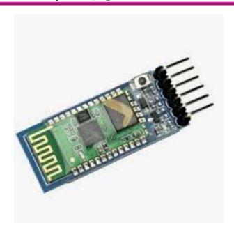
The HC-05 and HC-06 are common Bluetooth modules used with Arduino. They are capable of establishing wireless communication between the Arduino and other Bluetoothenabled devices. Bluetooth modules use the Serial Communication Protocol (UART) to communicate with the Arduino. This simplifies the process of sending and receiving data wirelessly. Some Bluetooth modules can be configured using AT commands, allowing users to set parameters such as the device name, baud rate, and pairing code.
