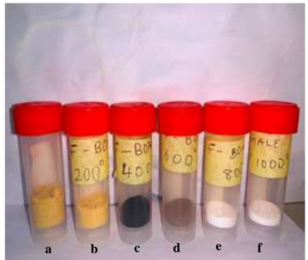
Fig. 5 Calcinated bone powder at different temperatures (a) raw bone powder (b) bone powder at 200°C (c) at 400°C, (d) at 600°C, (e) at 800°C and (f) at 1000°C.
