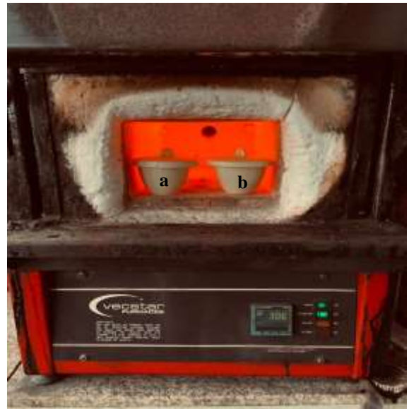
Fig. 4 Calcination process (a) Nanny femur bone powder in crucible (b) Billy femur bone powder in crucible
