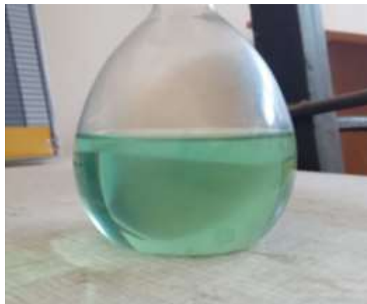
Fig.6. Filtrate solution obtained after zinc cake reductive leaching
