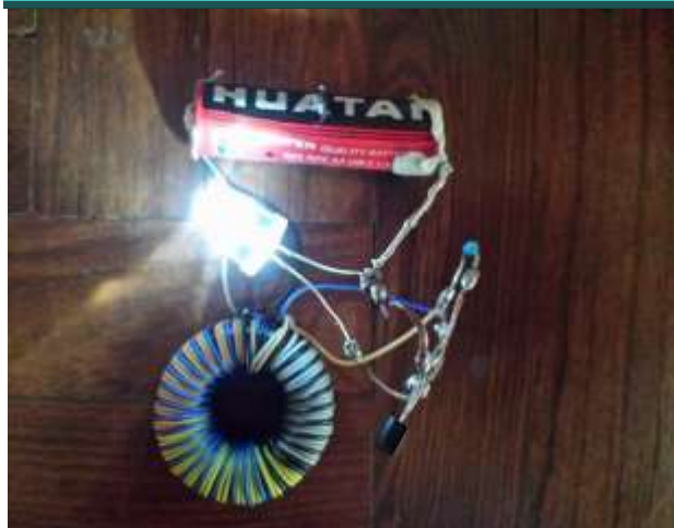
fig. 29. Installation of a single new battery of size AA with the circuit.
