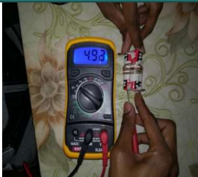
fig. 30. Measurement of the electromotive force of three new batteries combined of size AA.
