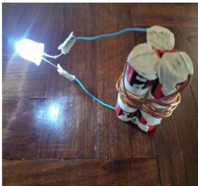
fig. 31. Direct power supply of an LED by three new batteries of size AA.
