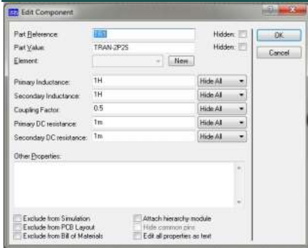
fig. 14. Adjustment of the resistance of the respective windings of the transformer for 1m \Omega .
