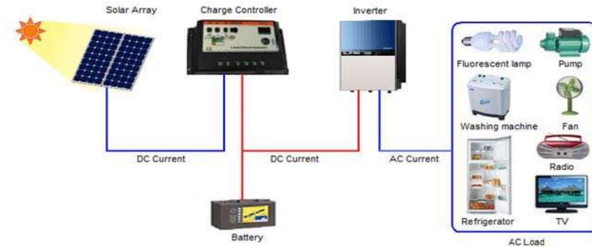
Figure 1: Schematic diagram of a typical domestic solar system (Zain et al. , 2019)
