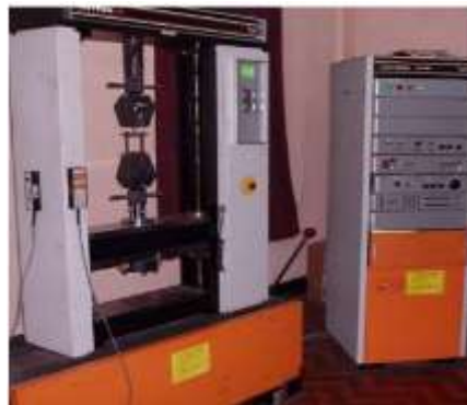
Figure 3.1. Experimental set up for three point bend test
