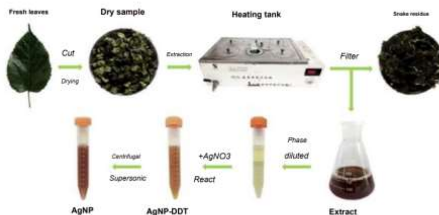
Figure 1. Flowchart of the extraction process of compounds in leaves and synthesis of silver nanoparticles
