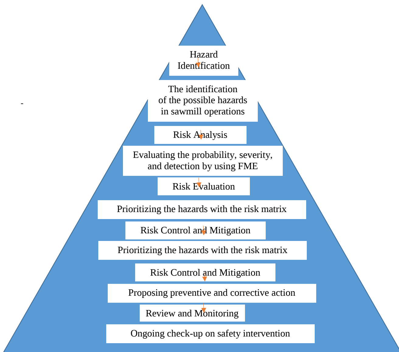
Fig. 1: Risk management Triangle and hazard evaluation using the FMEA
