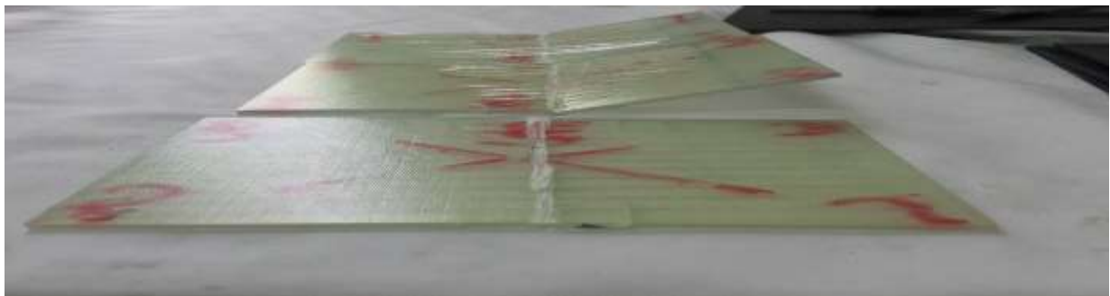
Figure 4. Photographs of specimens after impact showing visible surface indentation.
