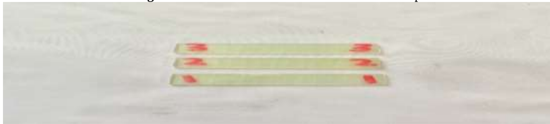
Figure 2. Cured E-glass/epoxy laminate before machining.
