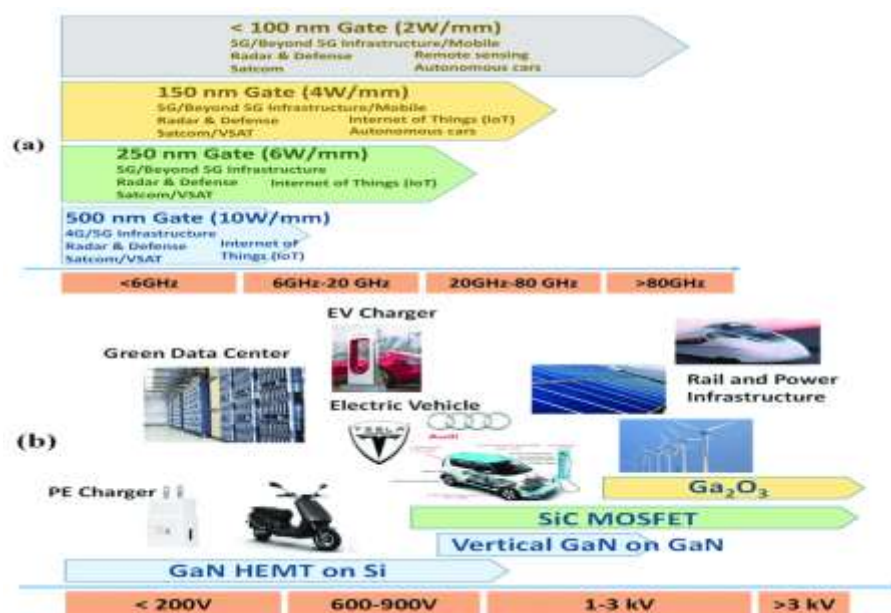
Figure 2: Development of GaN HEMTs Fabricated on Silicon, Silicon-on-Insulator, and Engineered Substrates and the Heterogeneous Integration ((a) A roadmap of RF GaN HEMTs technology. (b) A roadmap of Power GaN HEMTs technology) (Hsu, et al., 2021).
