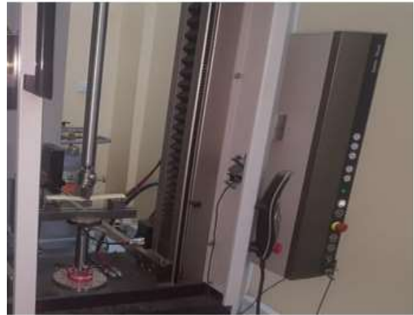
Fig 1: Zwick / Roell tester machine for 3 point bending tests.
