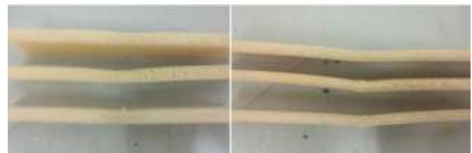
Fig 4: Shows cross-sectional view of specimen with 3 and 6 mm core thickness pending test.
