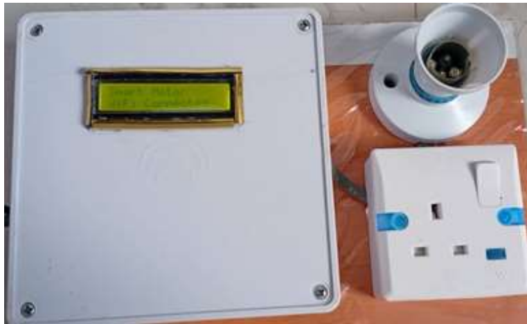
Plate 1: The developed IoT-based metering system with evaluating ports
