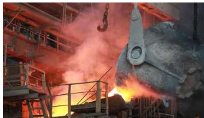
Figure 1. Liquid converter slag pouring into a reverberatory furnace in Metallurgical workshop of Copper smelter AMMC JSC
