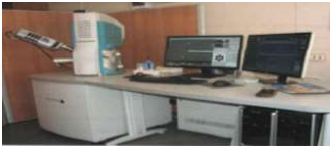
Fig. 2.1.4. TESCAN VEGA LMH electron scanning microscope with LaB6 cathode and Oxford Instruments Advanced AZtecEnergy X-ray energy dispersion microanalysis system.
