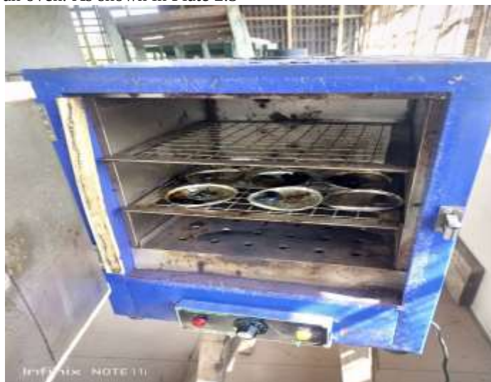
Plate 2.3: thermal treatment of medium cashew nut shells at 200, 250, and 300°C for 30, 60, and 90 minutes respectively
