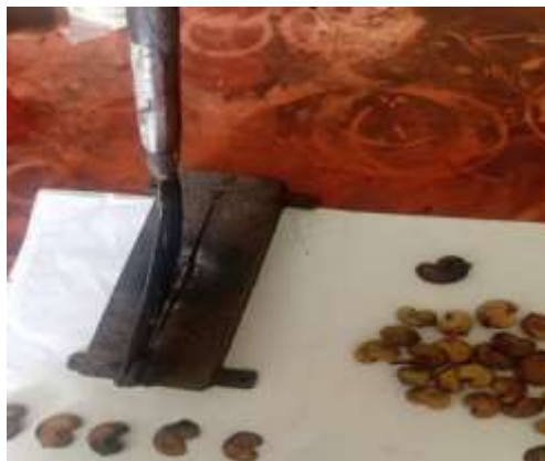
Plate 2.1: Manual cashew nut cracker
