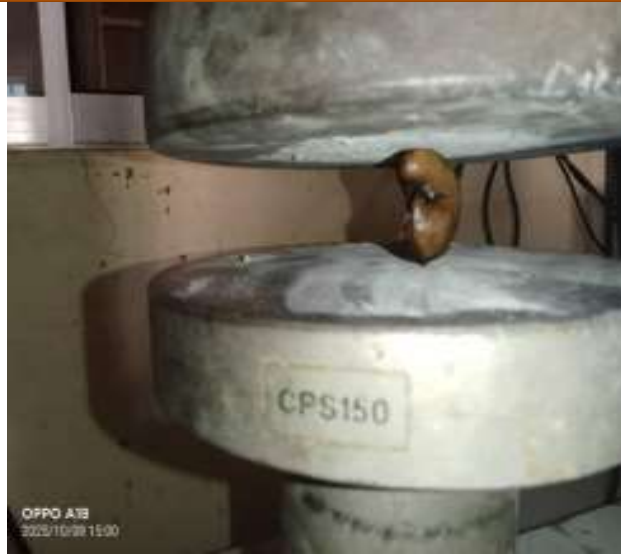
Plate 2.5: Determination of compressive strength and hardness of medium cashew nut shells
